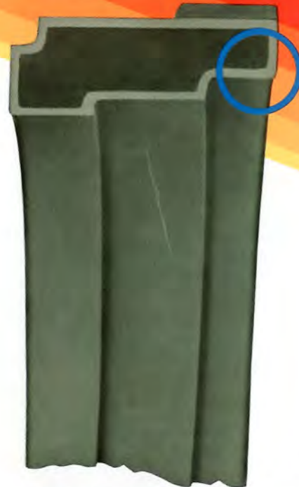
The broken cross-section of a typical TufMate seal ring shows the uniformity of surface conversion. This uniformity may be lacking in parts containing small holes, deep recesses or other configurations which restrict the circulation of silicon oxide vapor during the conversion process.
